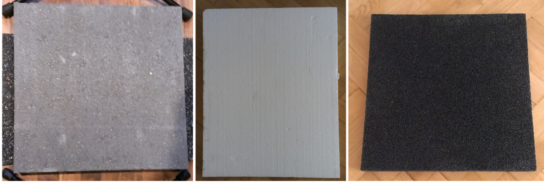
Figure 4.8: Samples for measurement; From the left side it is concrete, in middle is polystyrene and on the right side is rubber board
