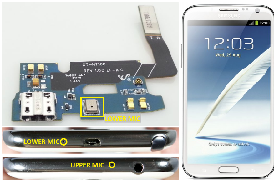
Figure 4.6: Samsung Galaxy Note 2, Microphone BLM15AG121SN1D
