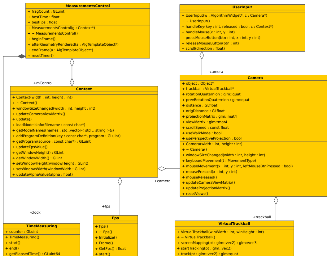
Diagram 3: Camera class is attached to UserInput to receive commands and is accessible via Context. VirtualTrackball is used in case of orbiting camera mode, walking mode is implemented as part of the Camera class. Fps and TimeMeasurements are used for measurements.
