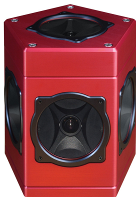
Figure 1.1: Image of the Ladybug3 camera.
