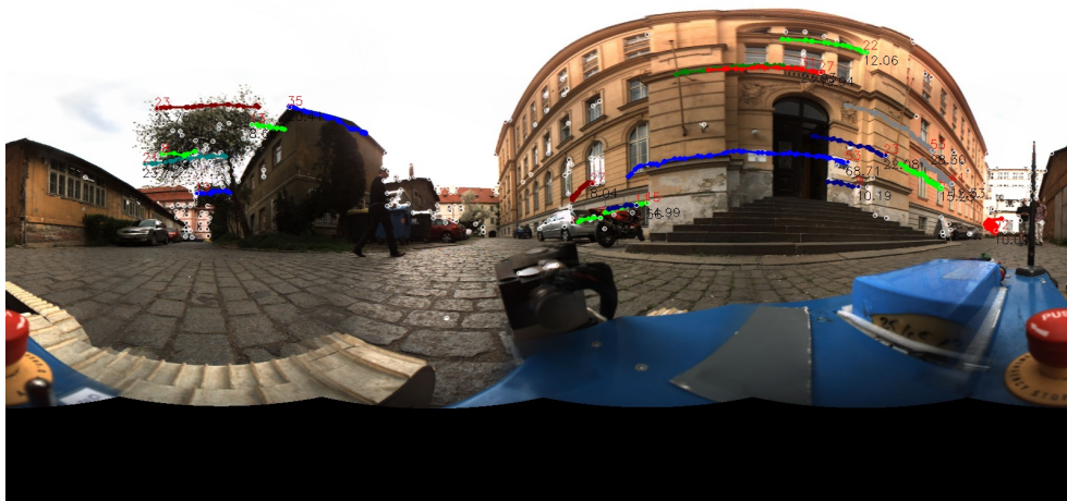
Figure 5.2: The Yard experiment: Picture from the ladybug3 recorded during the experiment. In the picture there are shown some key-points, which belongs to landmark. The red number is number of previous pictures, where exist correspondences to this keypoint. The black number is the landmark's apex angle.
