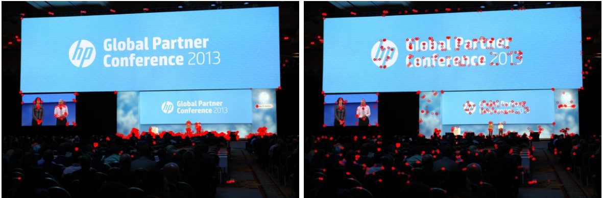
Figure 3.2 Non-maxima suppression. No keypoint (red) covers the HP logo after using standard ORB detector (left). Using spatial non-maxima suppression distributes the keypoints more uniformly (right).
