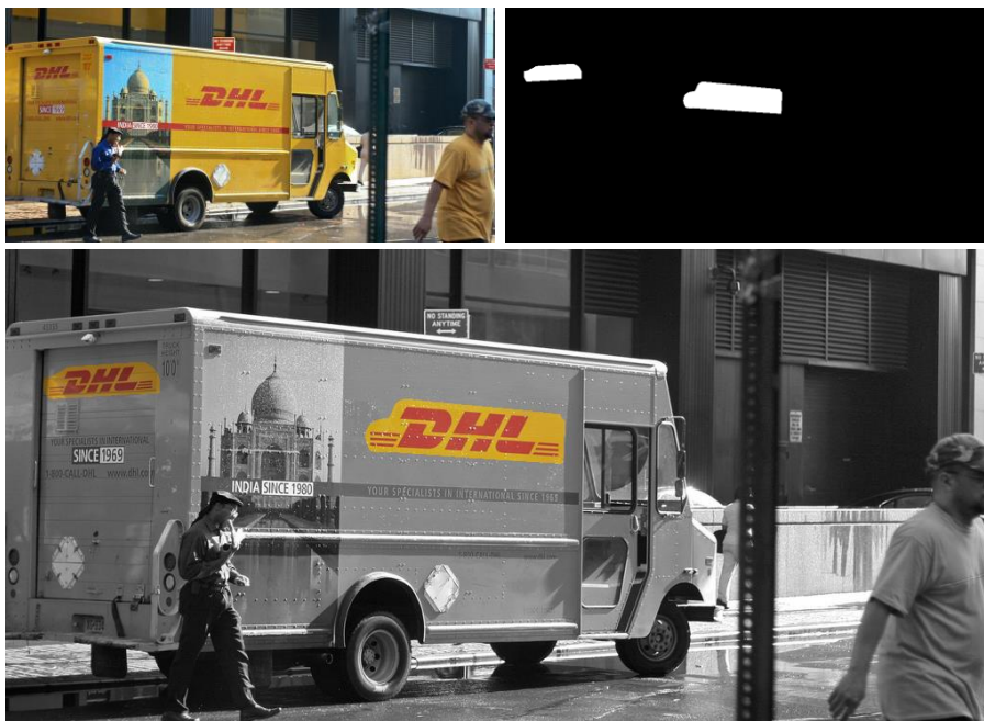
Figure 4.2 Pixel-level annotations. Original image (top left) and a mask of locations of logos (top right). Only keypoints which lie in the coloured areas are used for training (bottom).
