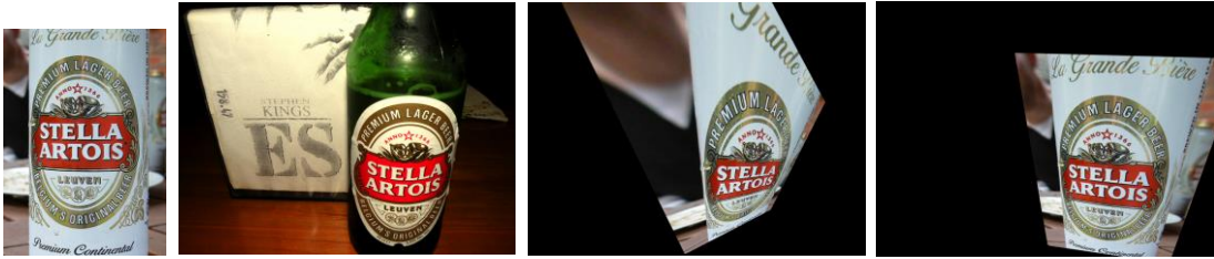
Figure 3.7 Deformed projection. Training image (left), query image (middle left), warped training image according to the transformation found without checking of the diagonals (middle right) and warped training image according to the transformation found after the diagonal checking (right).
