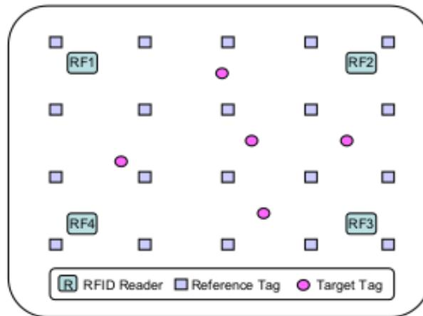
**Figure 2.12.** Example of LANDMARC set up presented in [10].
