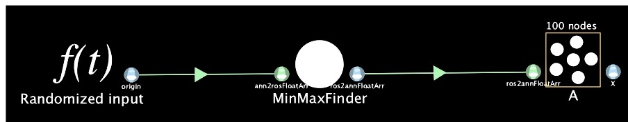
Figure 3.11: Example of simple hybrid system in NengoROS simulator. Neural Module (in the center) has inputs and outputs which correspond to the messages subscribed/published by the ROS node. The ROS node searches for the minimum and maximum value in the input vector of size 4. Neural Module is treated as an ordinary neuron (with more inputs/outputs) by the simulator. Note that multi-dimensional connections are shown as one line here.
