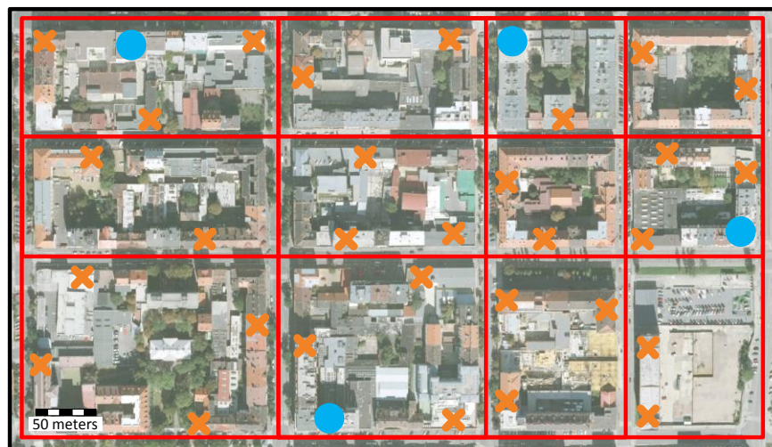
Figure 8: Simulation area in Prague, Czech Republic with position of microcells (blue circles), SCeNBs (orange crosses), and streets (red lines)
