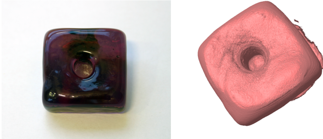
Figure 3.5: A transparent object (left) and its model obtained by the tomography. [171]
