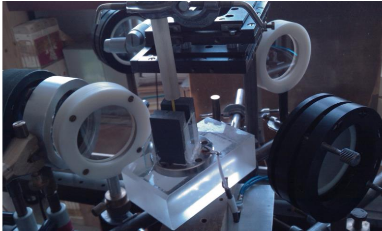
Figure 40 Experimental setup of the apparatus used for detection of pressure field around corona-like discharges in liquid water solution in a glass cuvette (top). Photograph of the Mach-Zehnder interferometer with the cuvette.
