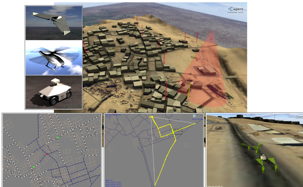
Figure 5.2: Tactical AgentScout simulator facilitates rich models of physical reality and supports physical mobility dynamics of robots, such as ground and aerial vehicles, be it fixed-wing aircraft, helicopters or various rotorcraft.
