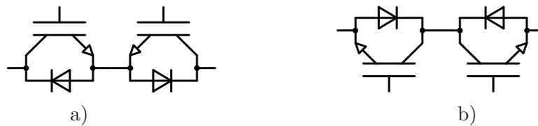
Figure 2.4. Bidirectional switch topology
