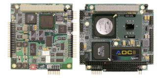
Figure 6.16. CPU module and ADC module
