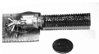
FIG. 3. The fluxgate gradiometer shown with 1-cent coin.
