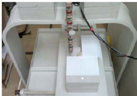
Fig. 8.1 – The gradiometer vertically placed above a non-magnetic bed, from [Platil 2013]
