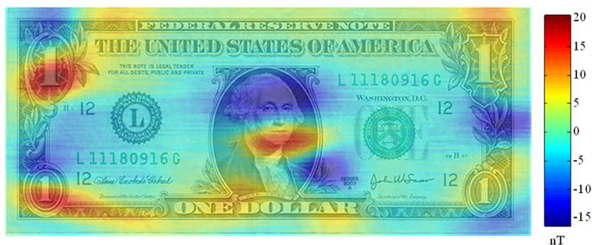
Fig. 6.4 – The mapped magnetic field gradient – 5 mm liftoff – above the 1 USD banknote. The 20 nT difference signal corresponds to 20 nT·mm -1 gradient. From [Pribula 2011].
