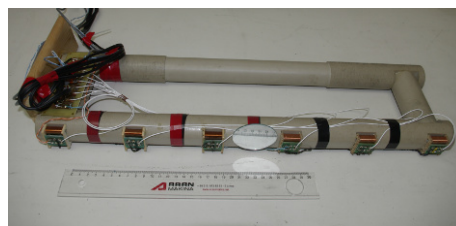
Fig. 8.2 – Detail of the 6-channel gradiometer (positioned horizontally). Z-direction is parallel to the 30-cm ruler.
