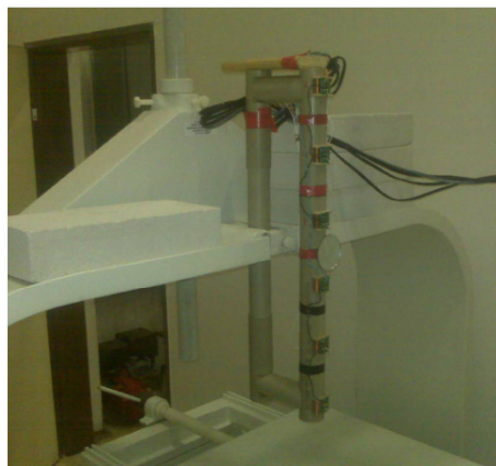
Fig. 1. The new robust 6-probe holder made of PEEK.
