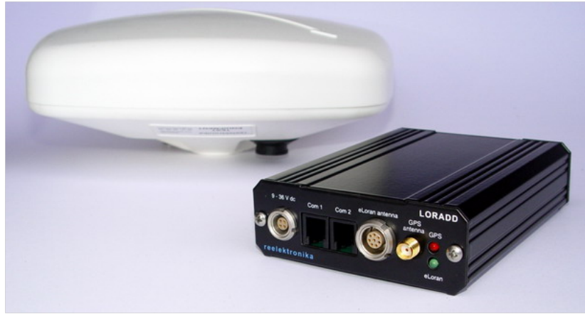
Figure 27: A combined eLoran H-field\GPS antenna and the Reelektronika LORADD eLoran receiver (photo courtesy of Reelektronika b.v.).
