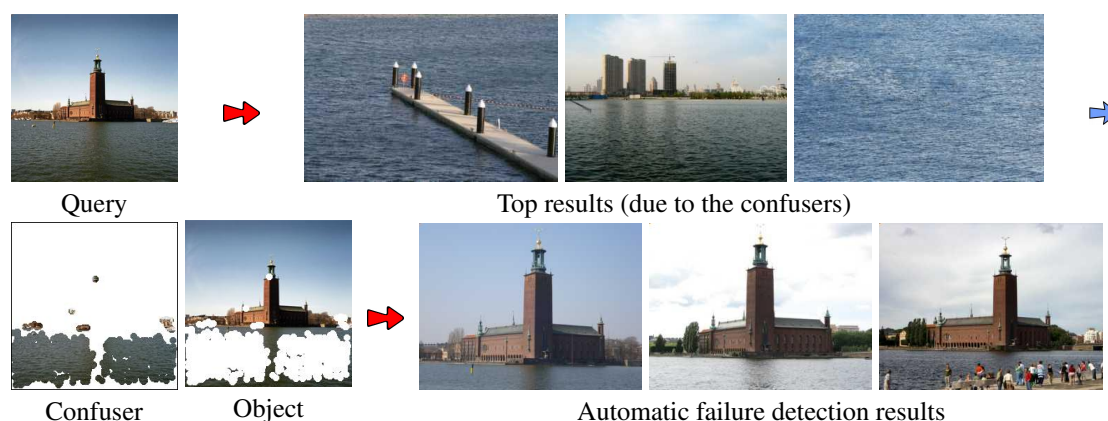
Figure 5.1: Automatic Failure Recovery : Initial retrieval results corrupted by confusing water features. The confuser model is learned dynamically. Successful subsequent query using the confuser model.
