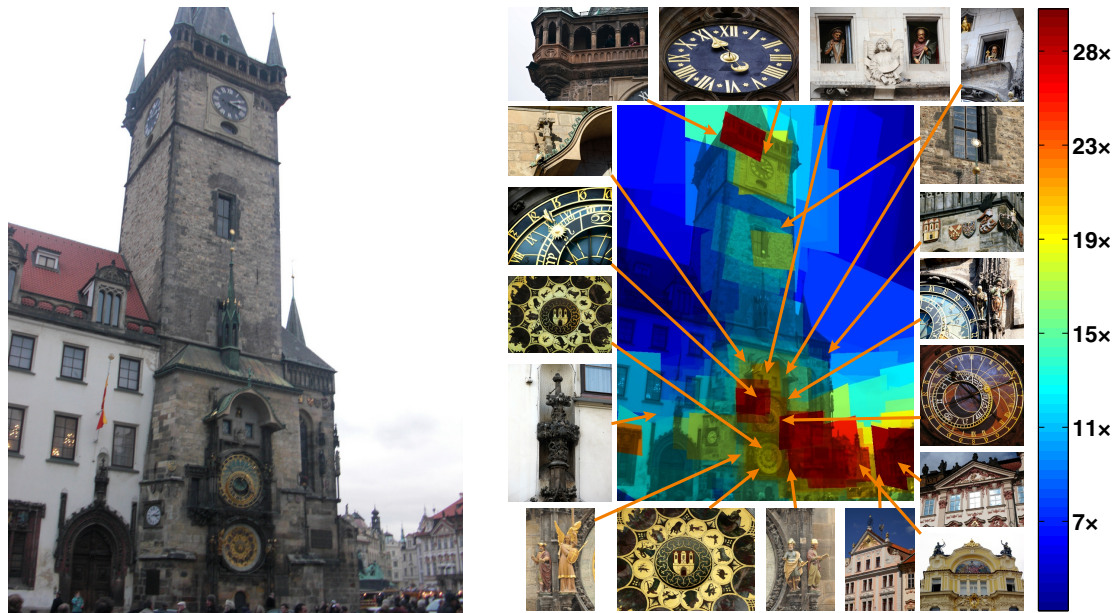
Figure 6.4: The “ Highest resolution transform ” (right, central part) color-codes the available zoom-in factor at each pixel. For the query (left), the maximum scaling factor is about 30; scaling factors are expressed as ratio of lengths. The retrieved detailed images are shown around the border together with links to the pixels they correspond to. Hovering with the mouse above the query image in the retrieval system interface the images with the highest resolutions could be shown. A dataset-supported superresolution-like functionality could be easily implemented.
