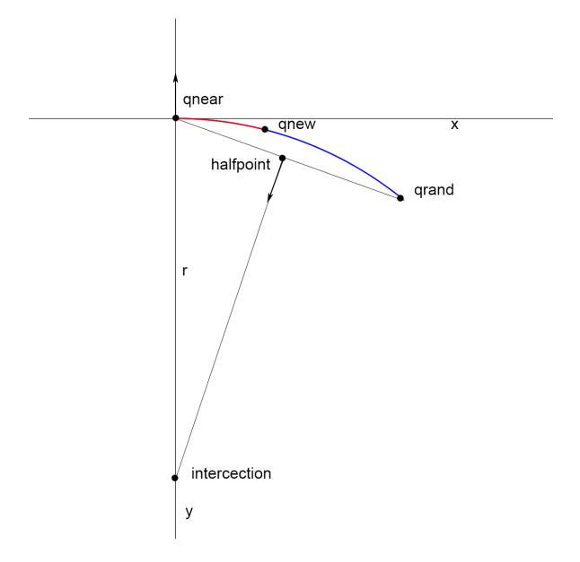
Figure 3.1: Computing control input.
