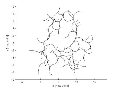
Figure 5.1: Example of generated RRT tree, after 300 iterations.
