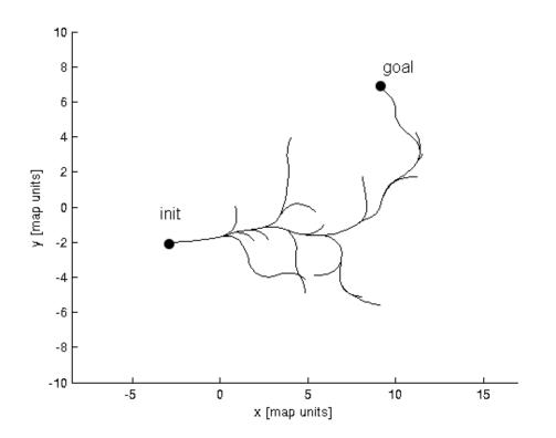
Figure 5.5: Exploration tree of T-RRT. In this case, T-RRT finds solution quickly without exploring other ideas, which is good behavior for next processing.
