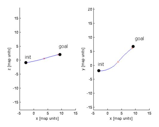
Figure 5.3: Reduced trajectory. Without obstacles, reduction result is adequate even for RRT.
