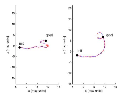
Figure 5.2: Trajectory generated by RRT. Trajectory is cluttered and crooked.
