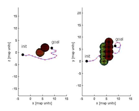
Figure 5.14: Initial trajectory. Initial trajectory leads under the obstacles.
