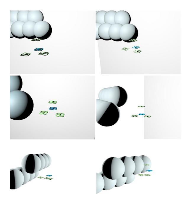
Figure 5.17: Visualization of a formation flying around obstacles. The blue quadrotor is leader and followers are green.
