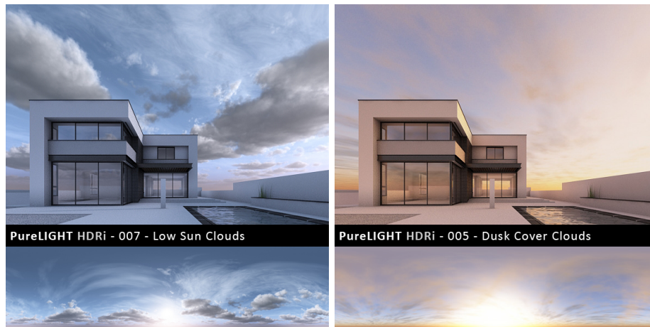
FIGURE 2.5: Example of IBL technique with diferent HDR sky dome panoramas. Source [35]
