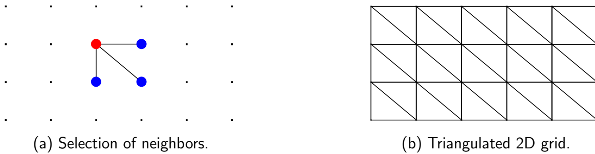
Figure 3.3: Triangulation of a 2D grid where the red dot represents the original point and the blue dots represent its neighbors during neighbor selection.
