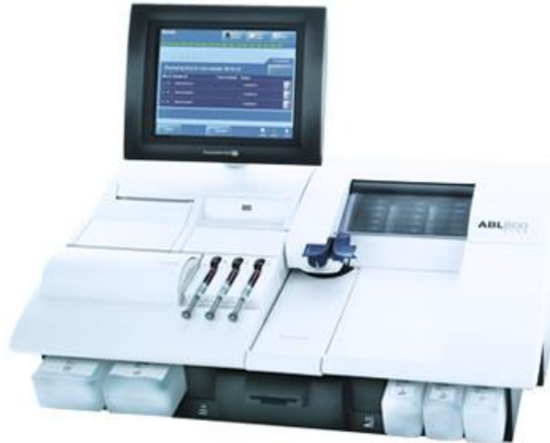
Figure 4 Automated benchtop blood gas analyzer [10]
