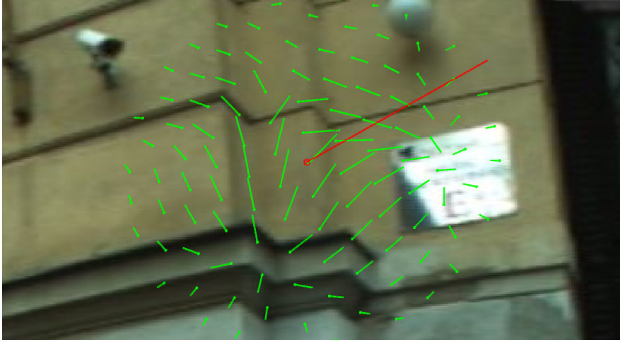
Figure 3.6 Unit gradient directions \mathbf{r} at sample points (green), weighted by their distance from the keypoint, and the resulting dominant direction \gamma (red). Gradient magnitudes used to determine \gamma are not visualized in this drawing.
