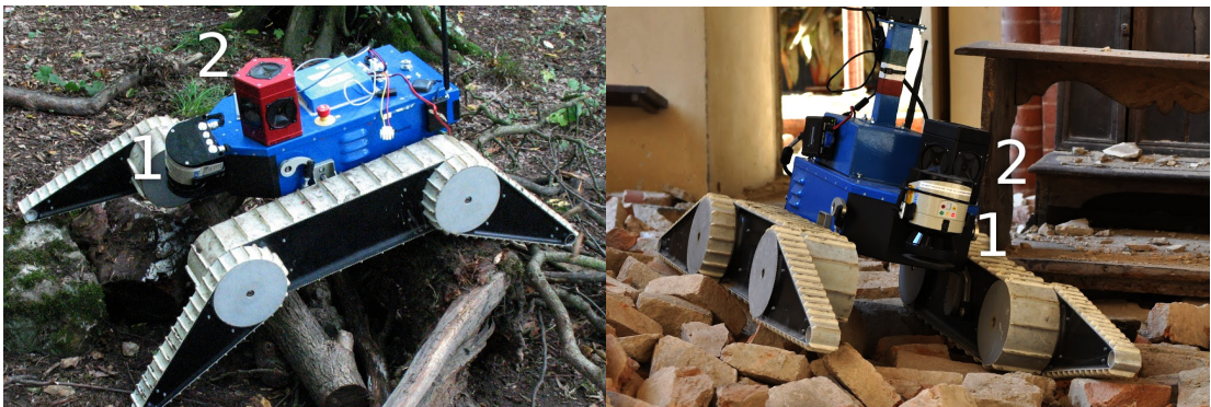
Figure 1.2 The NIFTi robot, featuring Sick LMS-151 laser scanner (1), and PointGrey Lady-Bug 3 omnidirectional camera (2). Images taken from [1, 4], respectively.
