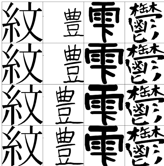
Figure 3.2: Examples of shape normalization performed on different images. First row: cropped original images fit into square; Second row: images after linear normalization; Third row: images after moment normalization.
