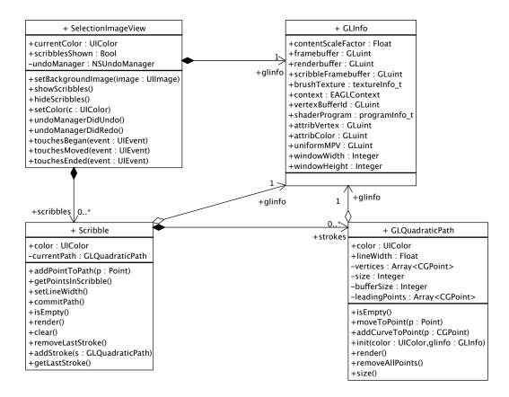
Figure 7.12. Scribble class diagram with GLQuadraticPath
