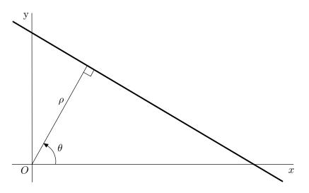
Figure 7.5. Polar representation of a line
