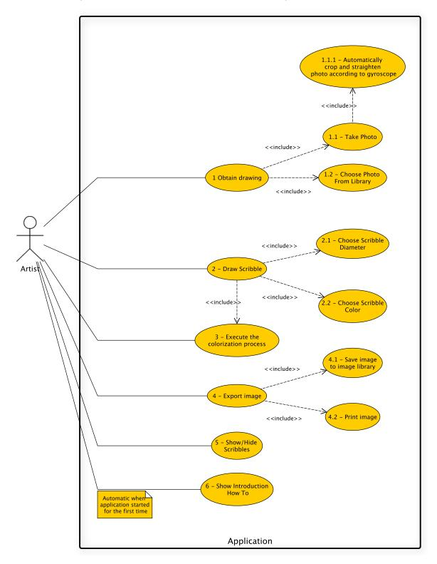
Figure 5.1. Use case diagram
