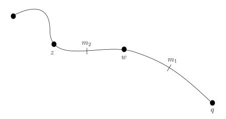
Figure 7.11. Quadratic Spline Interpolation
