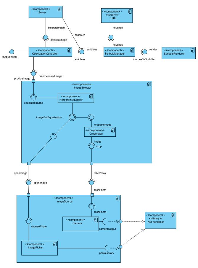
Figure 7.2. Application architecture component diagram
