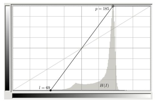
Figure 7.3. Visualisation of linear rescale of image intensities
