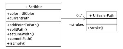
Figure 7.10. Scribble class diagram with UIBezierPath
