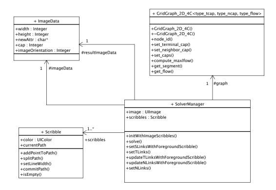
Figure 7.9. Solver manager class diagram
