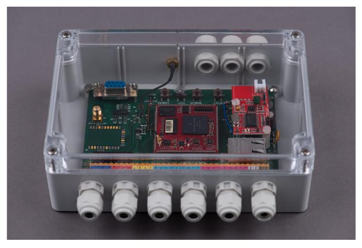
Figure 66. *BudkaControl* board covered in the covering box.
