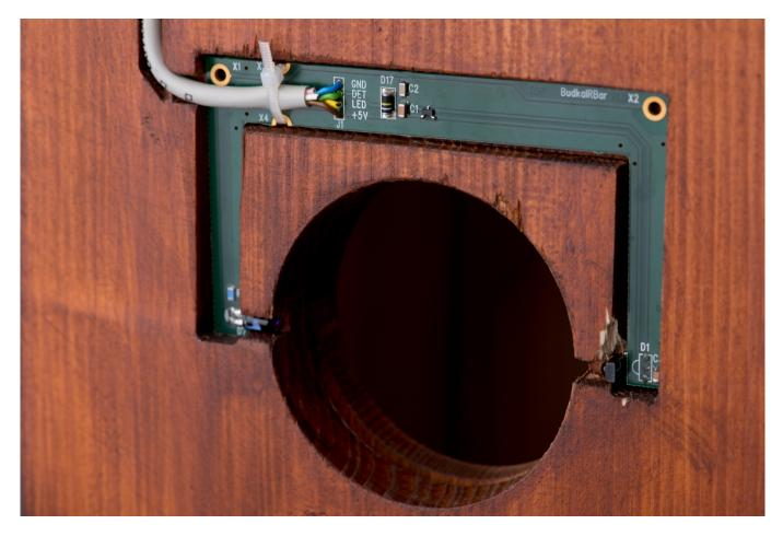
Figure 61. *BudkaIRBar* board installed in the nest-box.
