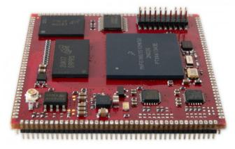
Figure 6. Photo of the SQM4-VF6-W module, the brain of the intelligent nest-box surveillance system. From [10].
