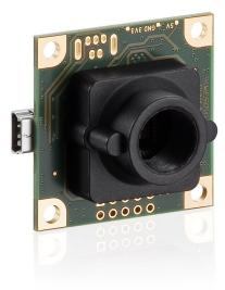
Figure 8. Photo of the UI-1541LE monochrome industrial camera. From [11].
