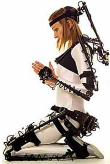
Figure 2.2: Mechanical motion capture system.[7]
