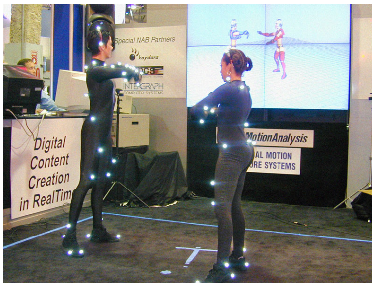
Figure 2.4: Optical motion capture system.[12]
