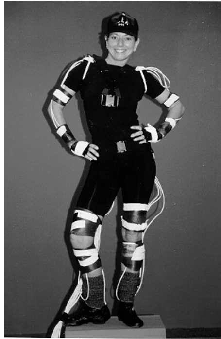
Figure 2.3: Magnetic motion capture system.[10]
