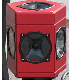
Figure 4.6: Ladybug 3 with 5 cameras placed horizontally in circle and one camera looking upwards for capturing omnidirectional images.
