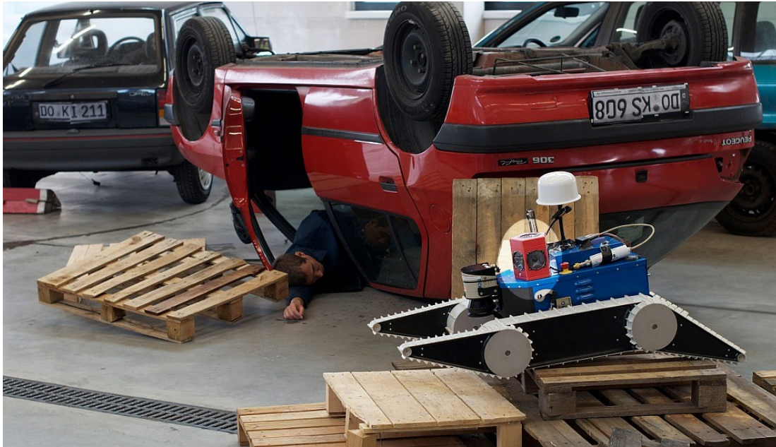
Figure 7.1: Our rescue robot with Ladybug3 omnidirectional digital camera on board. The camera has six 2Mpix chips and we want, among other tasks, to detect cars in five of them in real-time.
