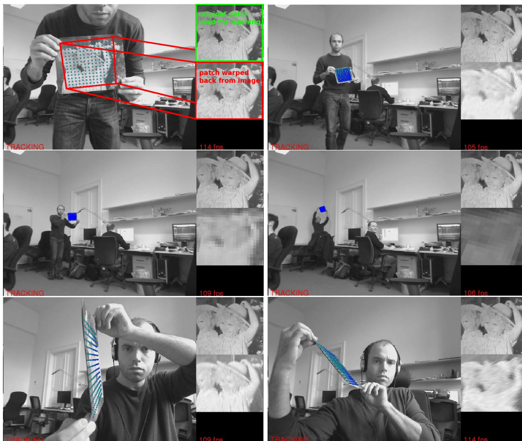
Figure 2.2: Here we see another result of our work. The tracker learned from a single image is marked by green rectangle. There is also the tracked patch warped back placed under the original patch for visual comparison (marked by red rectangle). Thanks to the incremental learning running during tracking the tracker is able to handle acute angle changes and significant changes in appearance caused by lower resolution of the tracked patch.
