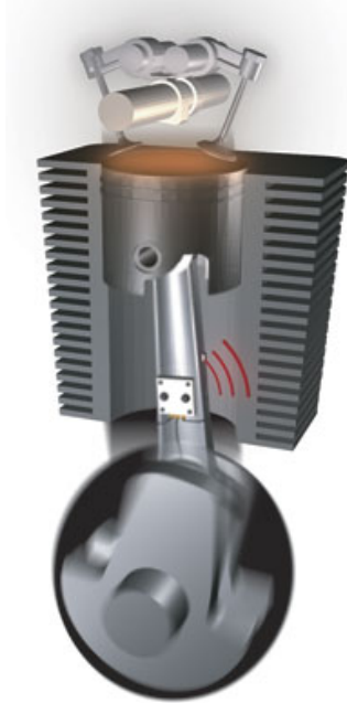
Figure 2.9: IRTs connecting rod wireless measurement technology [47]
