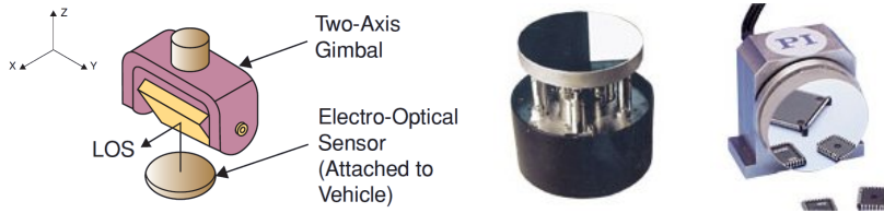
Figure 2.5: Left: The sketch of the fast steering mirror based stabilization principle. Image is adopted from [1].
