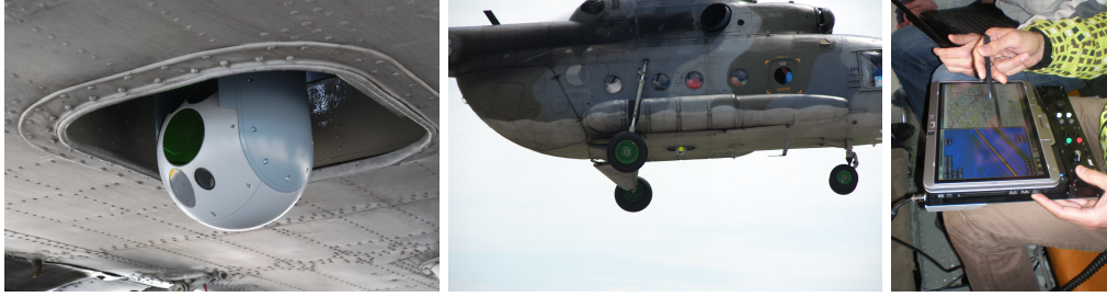
Figure 5.11: Left and Middle: Helicopter MI-17 with the platform S250 mounted underneath, Right: Touchscreen device used for operating the stabilized platform.
