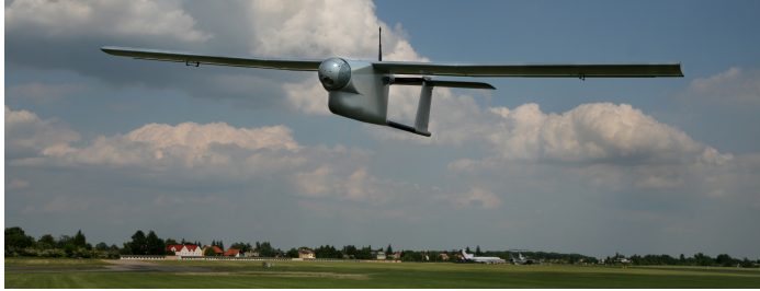
Figure 2.2: A double-gimbal platform mounted vertically (in the UAV nose) to allow stabilized observing of the target that is moving on the ground under the UAV. Singular point is thus moved to other location — horizon in this case.
