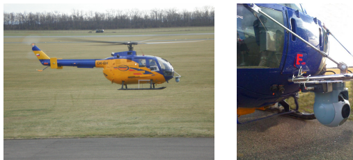
(b) The inertially stabilized airborne camera platform attached to a helicopter has to withstand significant vibrations caused by the carrier.
