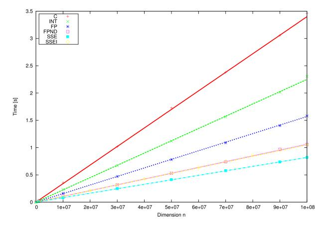
Figure 4.1: Vector multiplication with reduction timings - The meaning of lines is as follows. C - pure C implementation; INT - integer assembler implementation; FP - floating point implementation; FPND - floating point without division; SSE - floating point without division by means of SSE; SSEI - SSE implemented by means of Intel intrinsics
