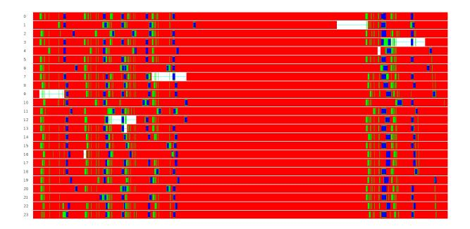
Figure 5.5: An example of the node workload for new architecture (n = 500, p = 24) - A detail close to the end. The meaning of colours remains the same as in 5.4. Even in the detailed view the nodes are busy almost all the time.
