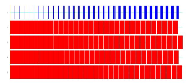
Figure 3.2: An example of the Node workload (n = 500, p = 5) - The graph of different processes utilization. The blue colour represents the master process and the red colour represents slave processes. The master process is idle almost all the time, while the slave processes are busy.
