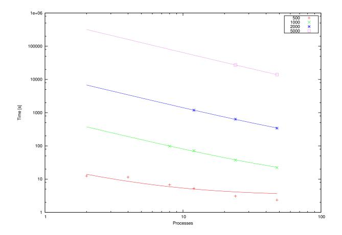
Figure 5.6: The linsolve parallel run timings in dependency on process count for different dimensions of SLE
