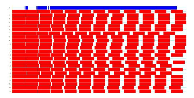
Figure 3.3: An example of the Node workload (n = 500, p = 24) where starvation is obvious - The meaning of colours remains the same as in 3.2. Master process is busy at later stage of computation and the slave processes starve (the gaps in red bars).
