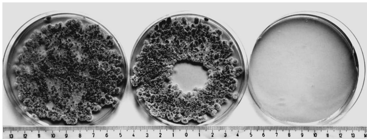
**Fig. 3.** Growth inhibition of *Eurotium amstelodami* by the combined treatment with the negative discharge and 10% hydrogen peroxide aerosol; control (left), exposed for 20 s (middle) and 180 s (right).
