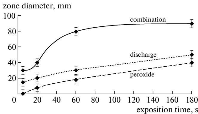
**Fig. 2.** The dependencies of inhibition zones diameter on the exposition time for solely negative corona discharge, solely hydrogen peroxide aerosol and those combination.
