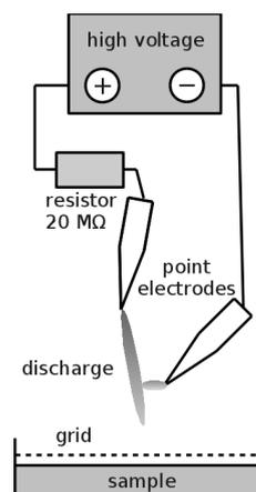
Fig. 1. Schematic arrangement of the device producing the cometary discharge with the grid. Objects are not in scale.
