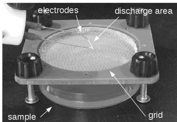
Fig. 2. The arrangement of the device producing the cometary discharge with inserted grid.
