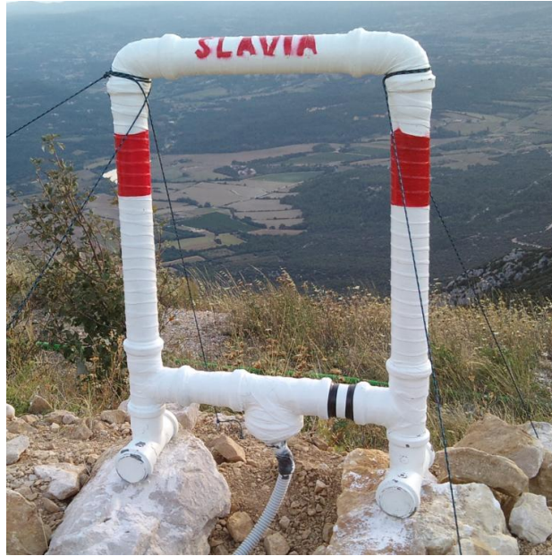
Fig. 51 Antenna loop type SLAVIA (Shielded Loop Antenna with a Versatile Integrated Amplifier)
