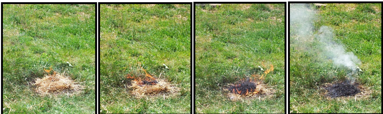
Figure 6.16: Burning of the straw fire 1 in 4-picture time series. Fire size 25 \times 25 cm.
