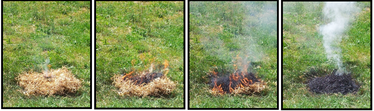
Figure 6.14: Burning of the straw fire in 4-picture time series. Fire size 50 \times 50 cm.
