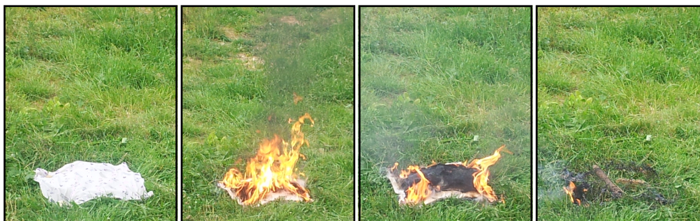
Figure 6.8: Burning of the gasoline fire in 4-picture time series. Fire size 50 \times 50 cm.
