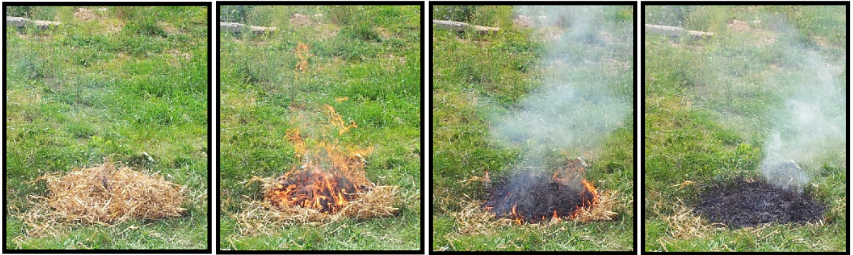
Figure 6.20: Burning of the straw fire in 4-picture time series. Fire size 60 \times 60 cm.
