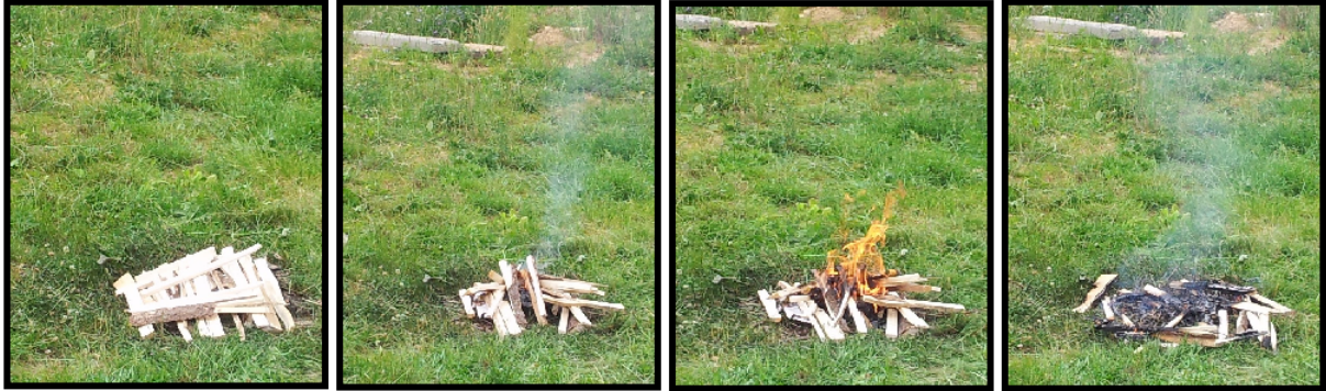
Figure 6.12: Burning of the wood cellulosic fire in 4-picture time series. Fire size 50 \times 50 cm.
