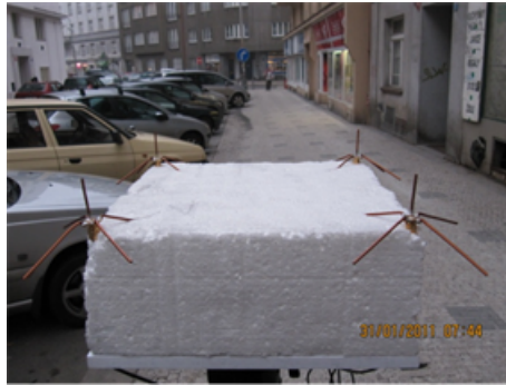
Figure 3.2: Receiving antenna arrangement at street level.
