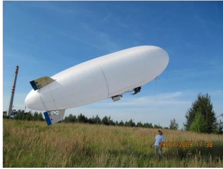
Figure 3.1: Remotely controlled airship used in measurements
