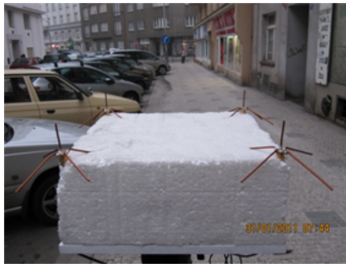
Figure 4.4: Receiving antenna arrangement at street level.
