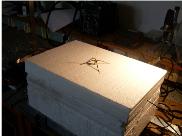
Figure 4.2: A quarter-wave monopole with rod ground plane used as a transmitter antenna
