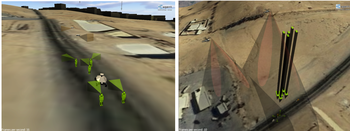
Figure 6.3.1: The ground forces (green) supported by the robotic team (2 small VTOLs – orange view prisms, 2 small VTOLs – red view cones, 1 UGV – brown four-wheeled car) in the simulated urban environment.
