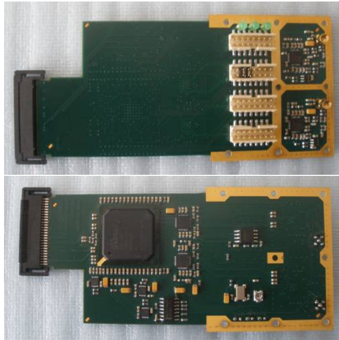
Figure 2.3: The Witch Navigator - ExpressCard PCB photos
