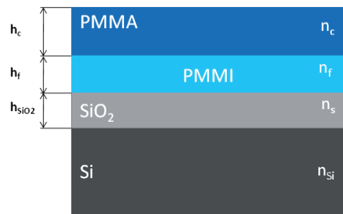
Fig. 3. Scheme of the PMMI optical planar waveguide.
