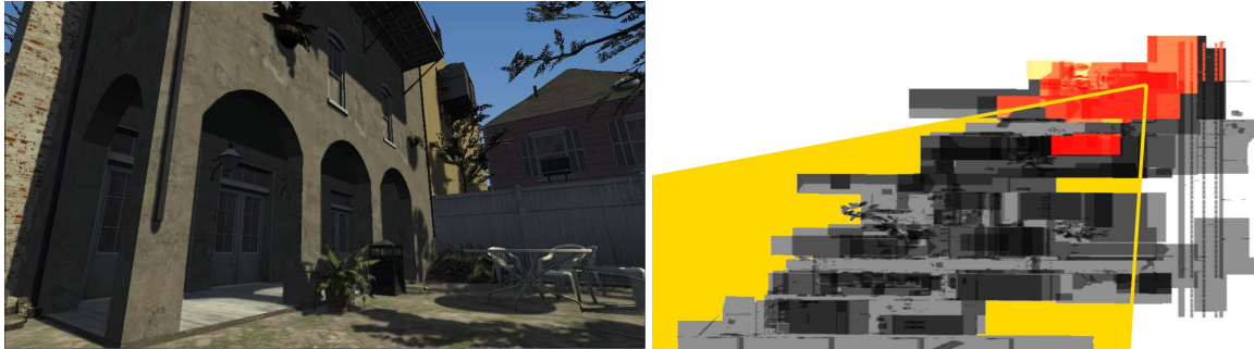
Figure 1: (left) A view of a game scene rendered with shadows. (right) Shadow map with shadow casters rendered using a naive application of occlusion culling in the light view (gray), and shadow casters rendered using our new method (orange). The view frustum corresponding to the left image is shown in yellow. Note that for this view our shadow caster culling provided a 3x reduction in the number of rendered shadow casters, leading to a 1.5x increase in total frame rate. The scene is a part of the Left 4 Dead 2 game (courtesy of Valve Corp.).
