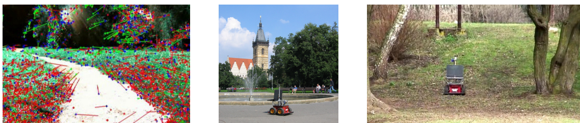
Figure 11: Examples of the detected landmarks, matching of the current and previously learned landmarks and outdoor environments where the navigation method provides reliable autonomous navigation.
