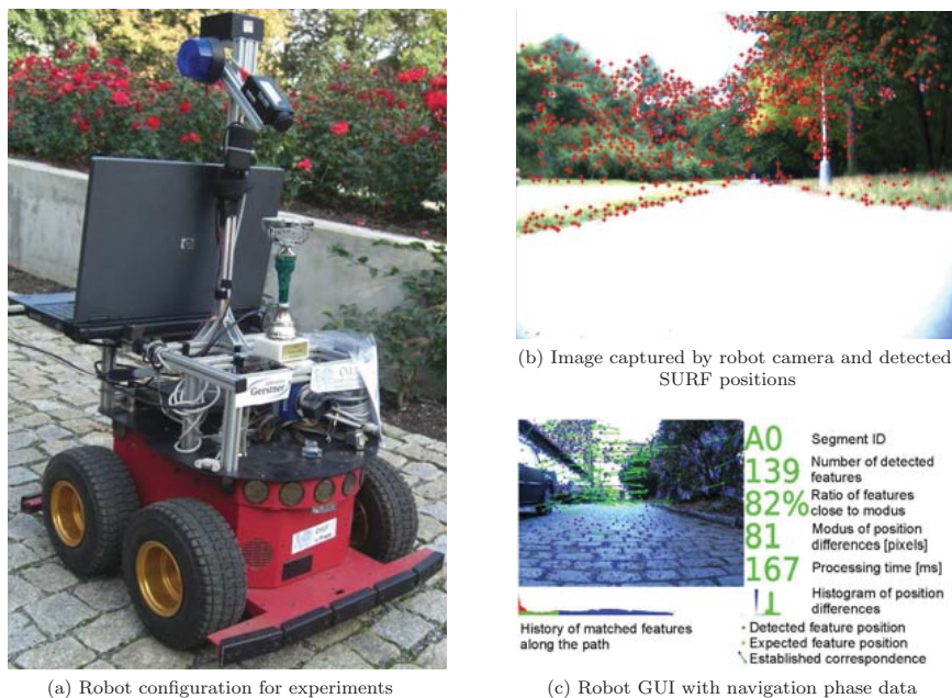
Figure 1. Robot platform, detected features, and navigation graphical user interface (GUI).
