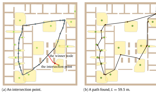
Fig. 5. Examples of an intersection point and a path found using the attraction algorithm variant, blue disks are nodes. (For interpretation of the references to colour in this figure legend, the reader is referred to the web version of this article.)
