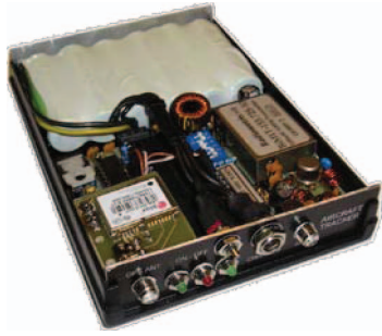
Figure 4. Transceiver Developed for Aircraft Tracking
