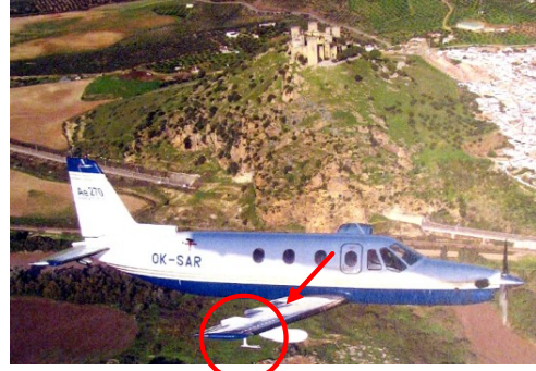
Figure 1. Placement of an AOA and AOS probe
