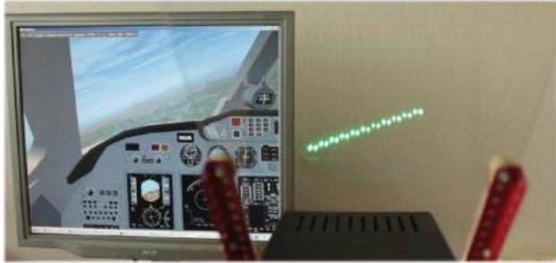
Fig. 14. Artificial Horizon Depicted by a HeadUp display using 2D array of bright LED diodes
