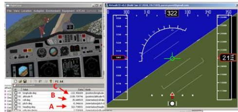
Figure 8. Final Instrument Developed by Students and Connected to the Flight Gear Simulator (comparable with Fig. 2).
