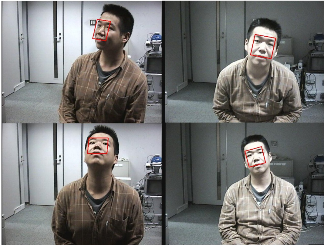
Figure 8.8: Examples of face tracking results. The red rectangle depicts SLLiP tracker aligned on human face.
