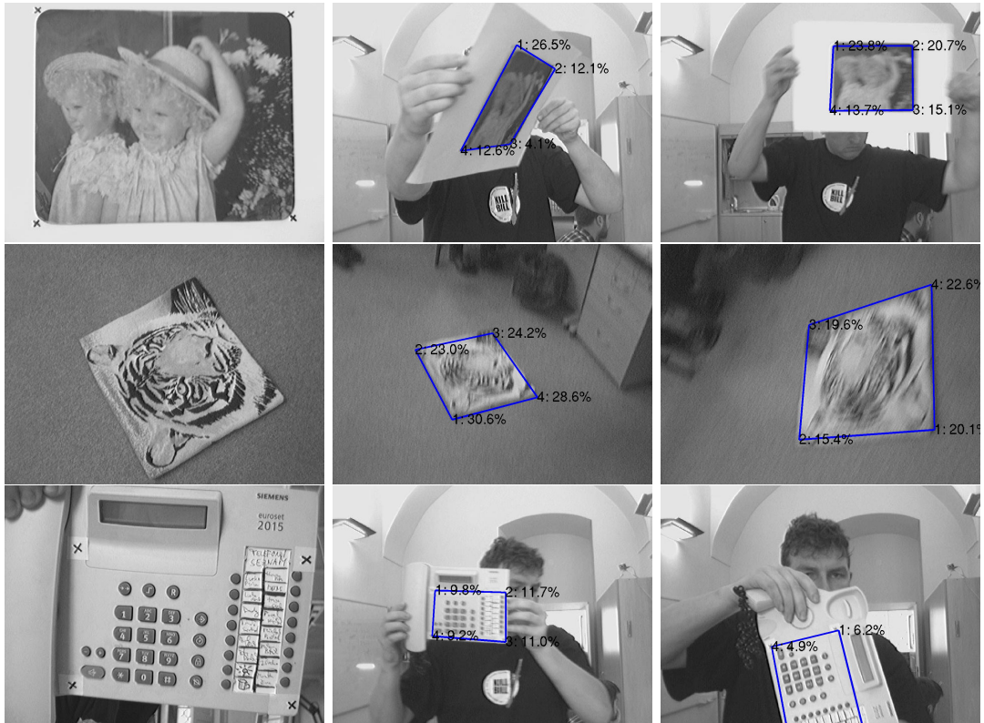
Figure 6.4: The left column shows images used for training. The middle and right columns demonstrate some successfully tracked frames with a strong motion blur from the testing sequences. The blue rectangle delineates the object. Percentage values in corners are current corner speeds related to the current size of the object upper edge.
