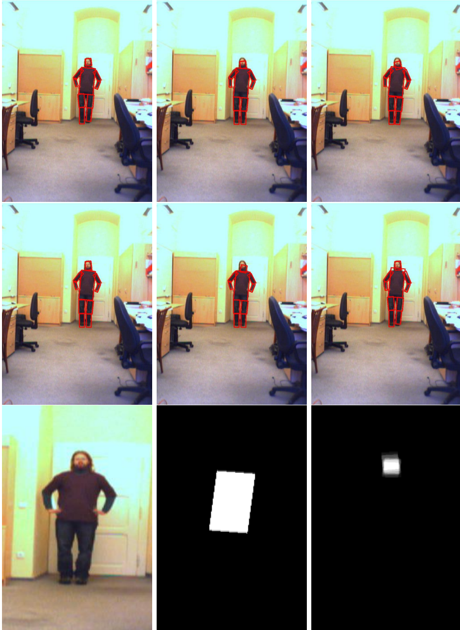
Figure 3.9: Examples of sampling from the posterior probability. The torso is sampled the same often in this case. The position of the head is different in each sample. The bottom row shows Frequency of occurrence of the parts normalised to the interval from 0 to 1. Left: original image. Middle: frequency of the occurrence of the torso. Right: the head occurrence frequency. The torso is sampled in a similar position in all the samples.
