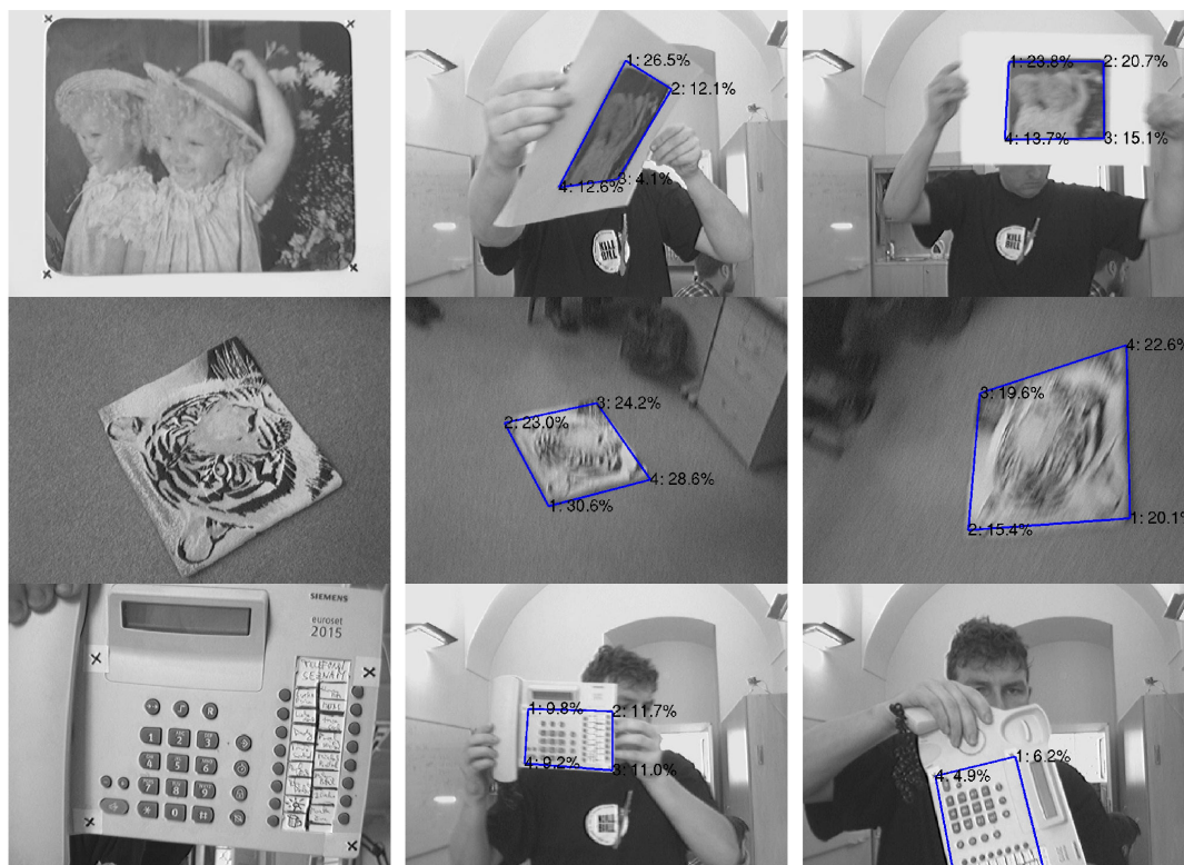
Figure 5.14: Ground truthed sequences: Left column shows images used for training. The middle and right columns demonstrate some successfully tracked frames with a strong motion blur from the testing sequences. The blue rectangle delineates the object. Percentage values in corners are current corner speeds related to the current size of the object upper edge.
