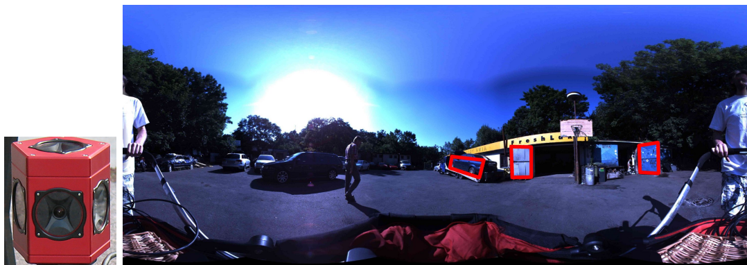
Figure 9.1: Omnidirectional high resolution image (12 Mpx) captured by Ladybug 3 camera (left). Three objects are marked.
