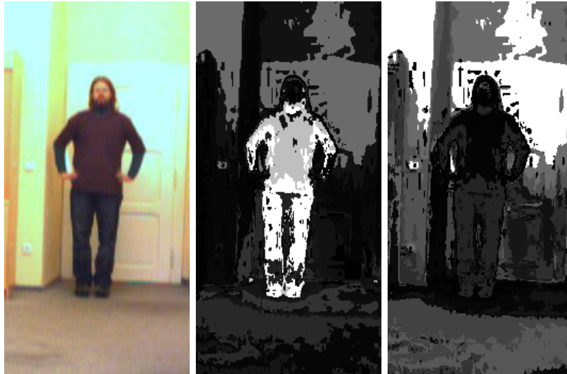
Figure 3.7: Initialization of the Graph Cut algorithm. Left: the original detection window. Middle: the probabilities that pixels belong to the foreground. Right: probabilities that pixels belong to the background. Black corresponds to 0, white to the maximal value.
