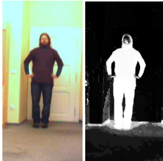
Figure 3.8: Probabilities of pixel belonging to the foreground. Left is the original detection window, right is the probability of each pixel belong to the foreground.
