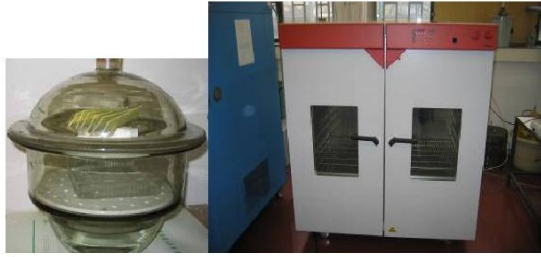
Fig. 4. Realization of humid and humid-heat stress. Samples were closed in an airtight container above the water level. This container was placed in the oven
