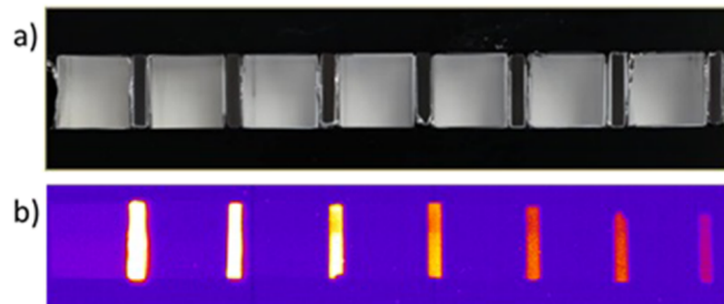
Fig. 2.14: a) picture of the calorimeter taken by the Andor Neo CMOS camera, b) camera image of scintillation light generated by a laser generated X-ray pulse [64].
