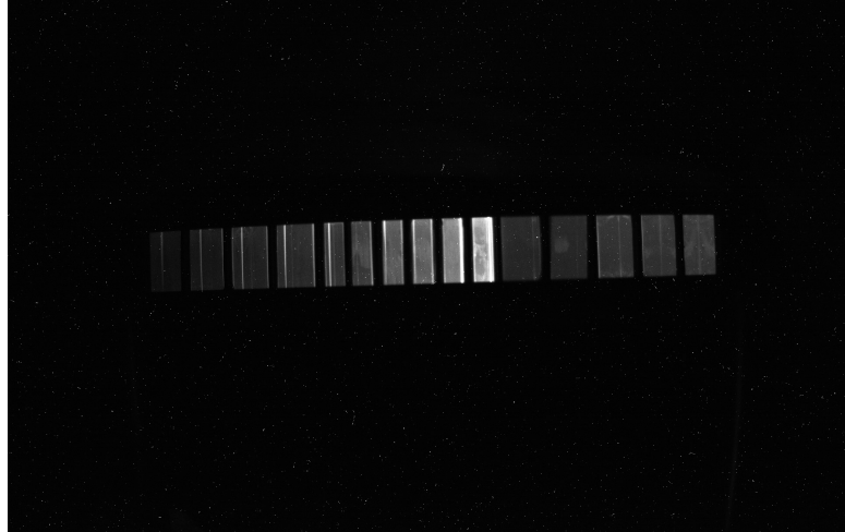
Fig. 6.8: Image taken during the Co-60 irradiation, the exposition time is 1000 ms, the gain is set to 30 db (same as during Cs-137 irradiation).
