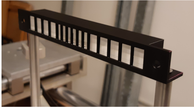
Fig. 4.6: Photo of the 3D printed calorimeter holder. Scintillators are placed in prepared slots, they are separated by a 1 mm PLA layer. The circular holes in the holder are used to attach the holder to other components (rods).
