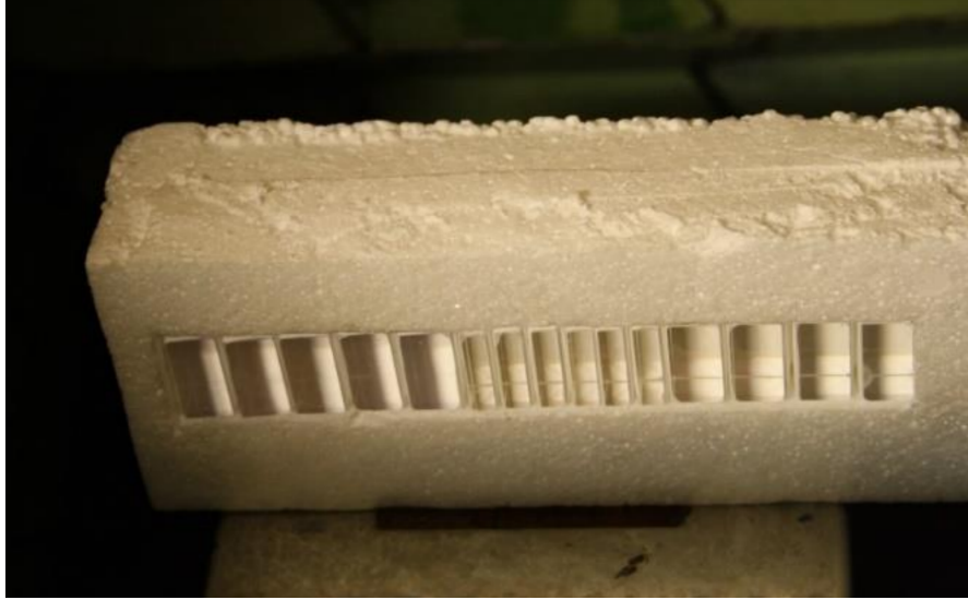
Fig. 4.4: Second version of the holder consisting of an expanded polystyrene block. This holder enables the camera to be placed from side. However, this solution is not cleanroom compatible and thus was never used at laser-plasma experiments.
