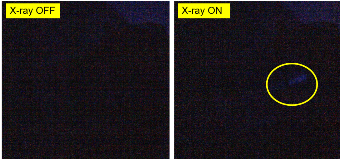
Fig. 4.8: Images taken by the Basler acA camera prior to the irradiation and during the irradiation. The gain of the camera and the exposure time is set to maximum. The faint glow of the first plastic scintillator is seen in the right picture within the yellow circle. It is evident that this camera does not have sufficient quantum efficiency to be used for the spectrometer.
