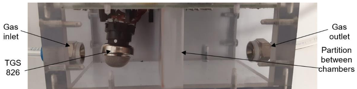
Figure 8. Photograph of conductivity sensor TGS 826 in test chamber.
