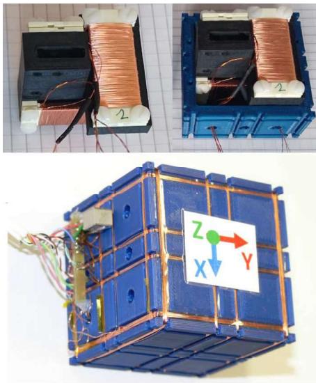
Fig. 4 Three 40 mm race-track-sensor-based triaxial fluxgate sensor head with a vector compensation of measured field (50 mm cube side).
