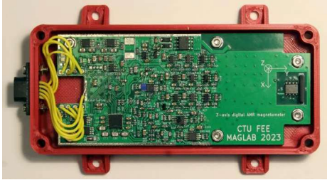
Fig. 8 Triaxial AMR magnetometer prototype.
