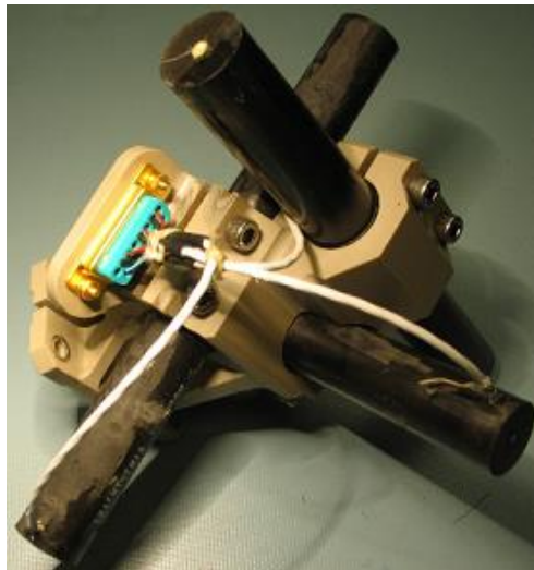
Fig. 4. Photo of 3-axis search coil magnetometer from THEMIS mission [NASA]
