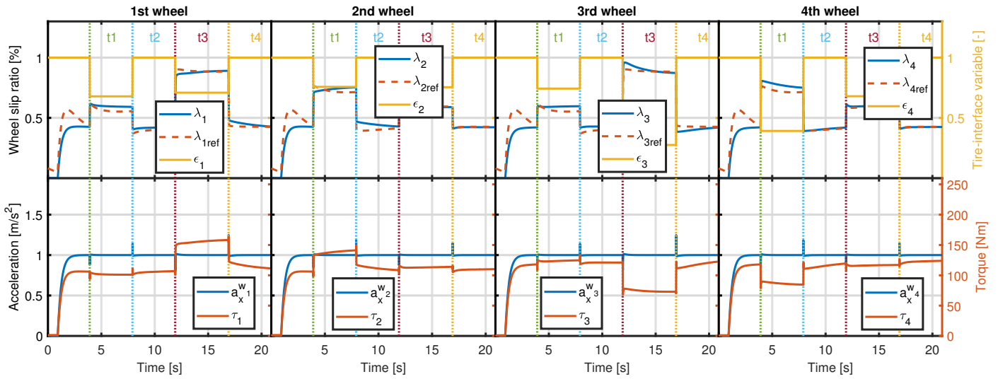
Figure 2.10: Wheels variables ( a_x^{w_i} , \tau_i , \lambda_i and \epsilon_i for each wheel) are shown here for the straight ride with \epsilon_i variation (described in Section 2.4.1). Simulation experiment is evaluated using the Matlab & Simulink model (see Section 2.1).
