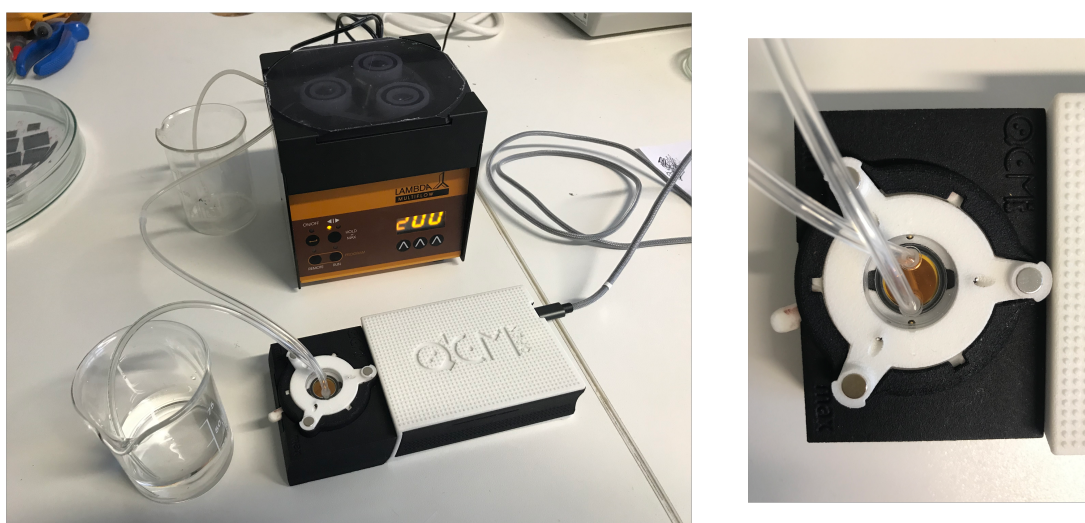
Figure 4.59: Measurement setup: OpenQCM Q^{-1} module with mounted QCM sensor connected to peristaltic pump
