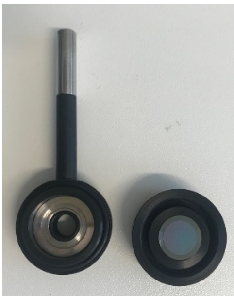
Figure 4.62: Home-made electrochemical QCM holder to contact BDD layer on top of QCM sensor
