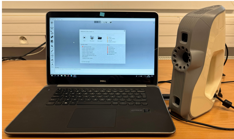
Figure 3. The used notebook and the structured-light 3D scanner Artec Eva.
