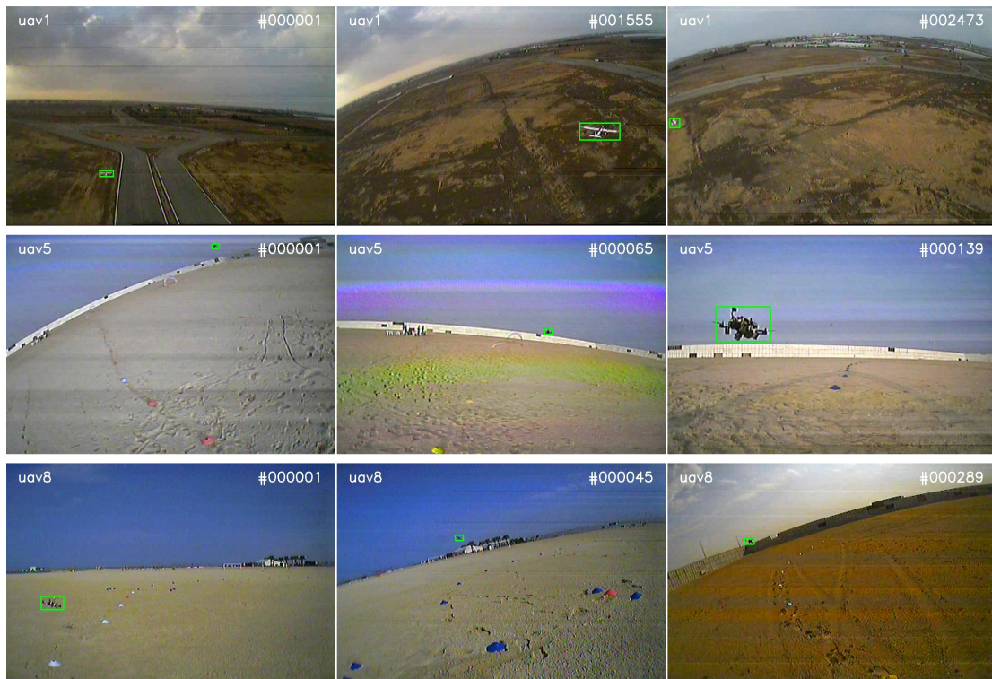
Figure 4.1. Frames of the selected sequences from the UAV123 dataset. The green bounding box indicates the ground truth annotation.
