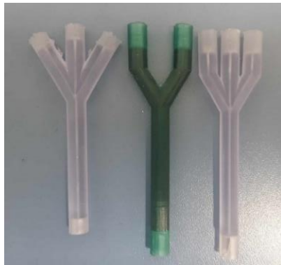
Fig. 12 The final 3D printed microfluidic devices
